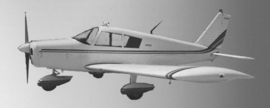
By selecting the  $\mathcal{L}_{\mathbf{Y}}$ - $\mathcal{C}_{\mathbf{on}}$  Rebuilding Co. 160 HP conversion, installed in your Piper Cherokee per STC SA00255SE you can expect some outstanding benefits in operating your Piper Cherokee 140/150. The  $\mathcal{L}_{\mathbf{Y}}$ - $\mathcal{C}_{\mathbf{on}}$  conversion was designed to make flying this aircraft even more enjoyable as well as economical..
