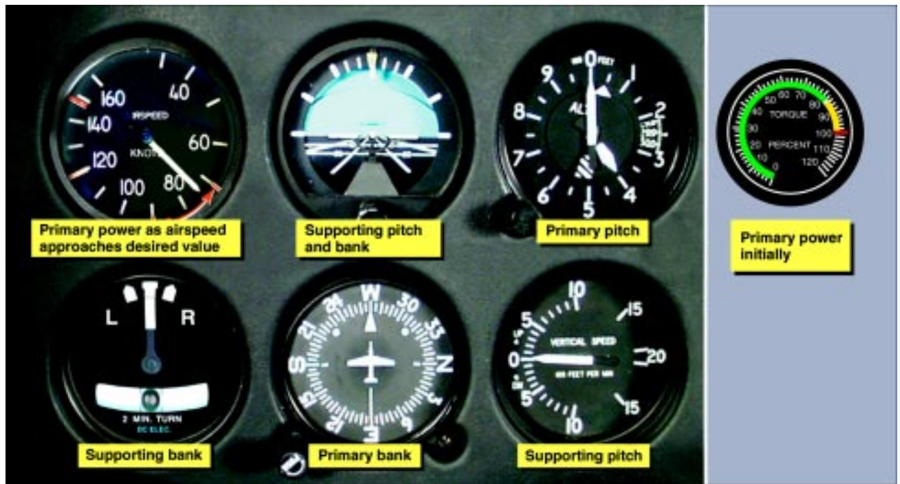
Figure 6-7. Flight instrument indications in straight-and-level flight with airspeed decreasing.
