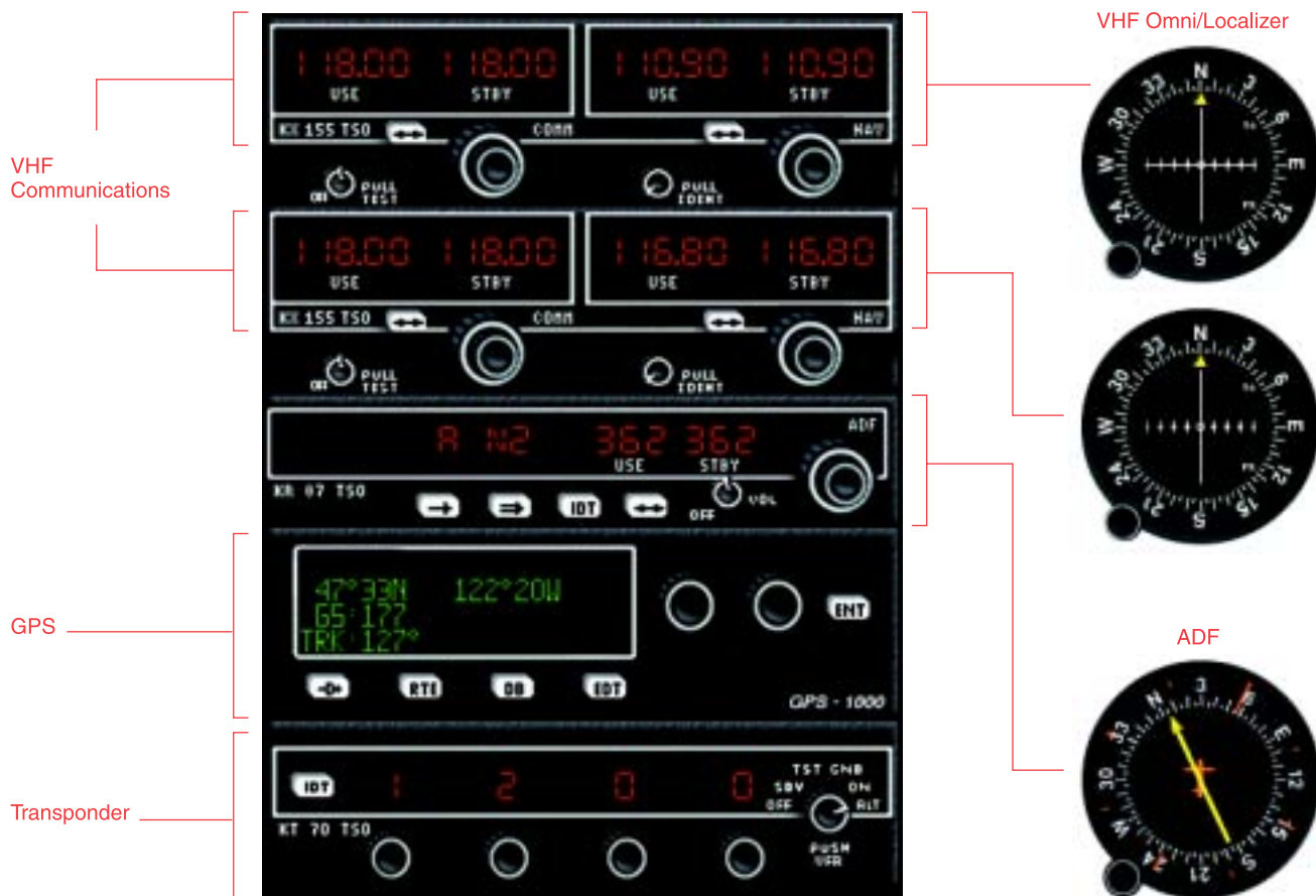
Figure 9-1. Typical NAV/COM installation.
