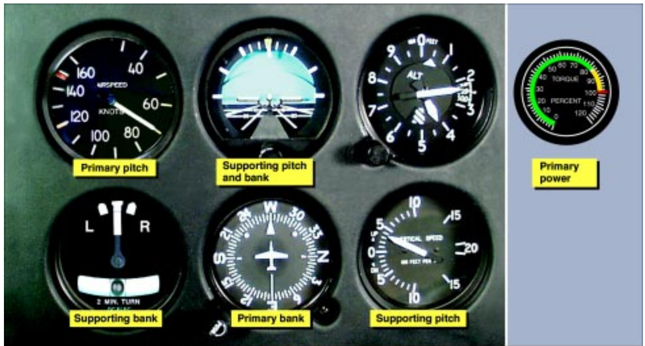
Figure 6-9. Flight instrument indications in a stabilized, constant-airspeed climb.
