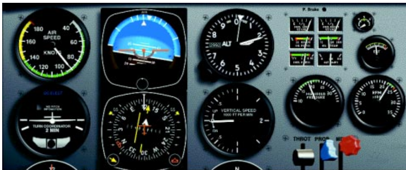
Figure 11-5. Vacuum failure — inoperative attitude and heading indicators.
